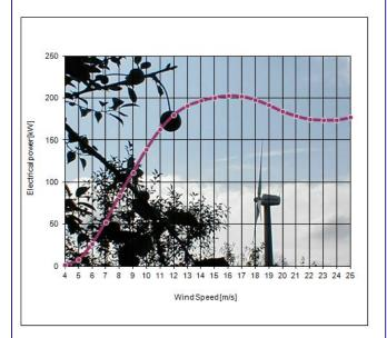
The power curve is for our 200 kW turbine, with a rotor diameter of 29 m, single generator and featuring Stall Regulation.
